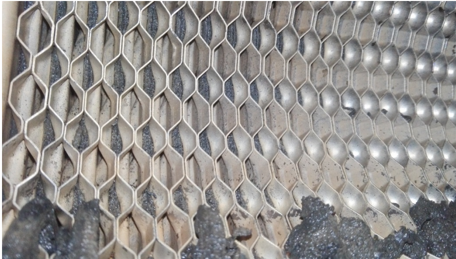
Figure 16 - Disintegration of the gasket caused by excessively aggressive cleaning agents
