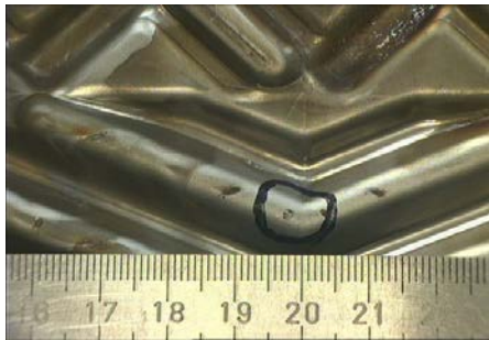
Figure 3 - Chafing locations at contact points
