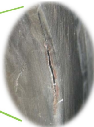
Figure 15 - Stress crack in the top plate. Product can therefore build up in the top plate, infecting the pasteurised end product
