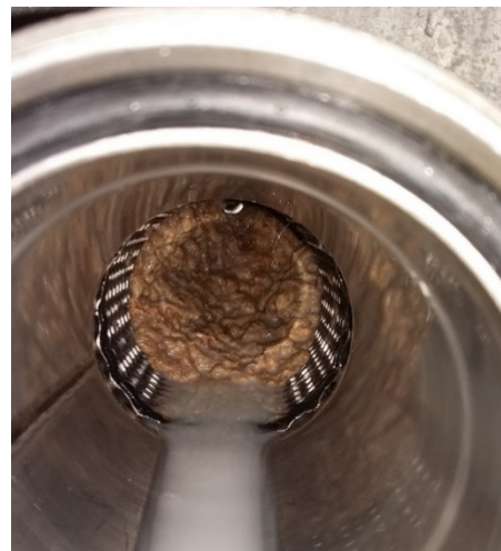
Figure 14 - Plate crack in the reversing group with product settlement
