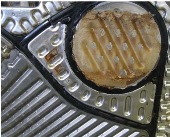
Figure 13 - Plate crack in the deflection plate. Resultant product deposits are not recorded by CIP cleaning
