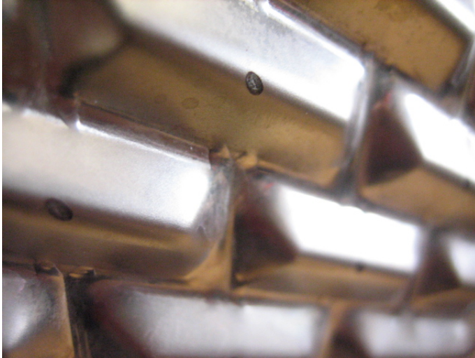
Figure 11 - Contact corrosion at the support points caused by resonances in the plate pack
