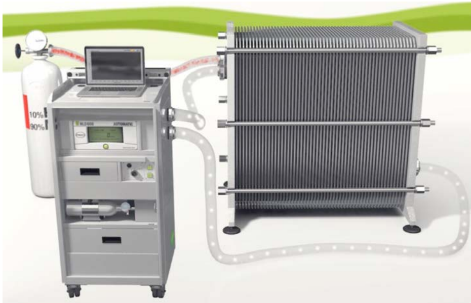
Figure 9 - Test layout during the plate test
